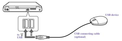
You can use the optional Sony USB mouse PCGA-UMS1 series with this computer. The USB mouse software driver is preinstalled in the computer. Therefore, you only need to plug the USB mouse into the USB connector.
